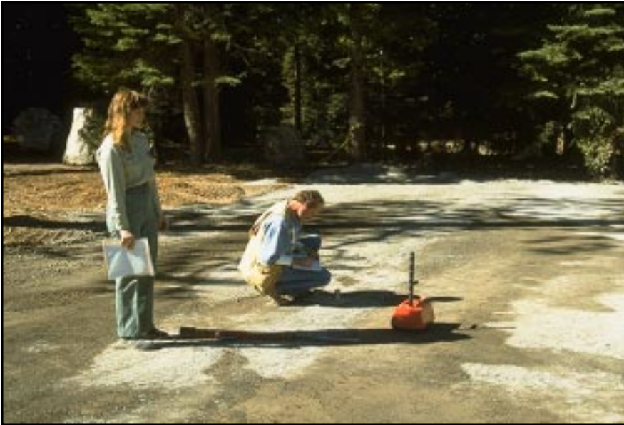
Photo 12.6 Here, a “nuclear gauge” is being used to check the density of aggregate. Use project construction quality control, gradation and density testing, etc., as needed to achieve the desirable materials properties for the project.
